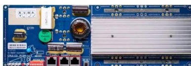
RS485 Communication between battery and sensors Baud rate: 9600bps RS485 Interface Communication between parallel packs or BMS and PC Baud rate: 9600bps
