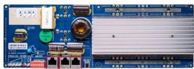
RS485 Communication between battery and server Baud rate:9600bps RS485 Interface Communication between parallel packs or BMS and PC Baud rate:9600bps
